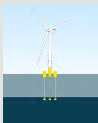
Tension Leg Platform
